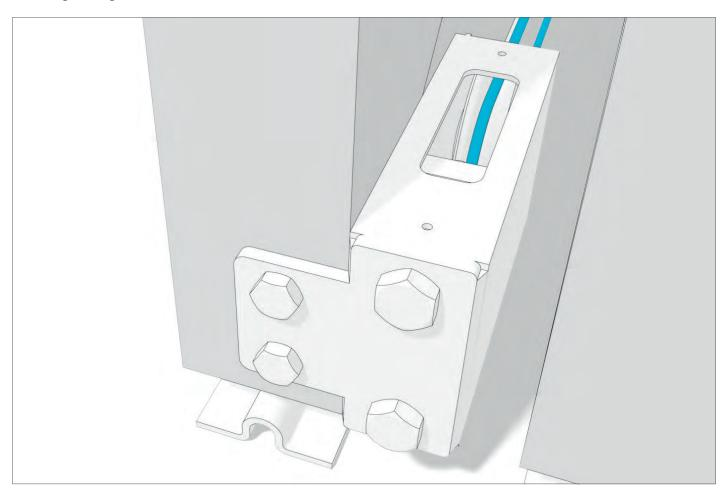
Close the sides of the pulley boxes with the supplied covers.
